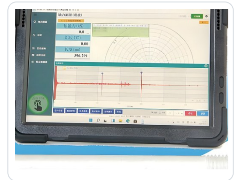
Measurement screen on the rugged terminal: axial force, temperature, bolt length and the live waveform
